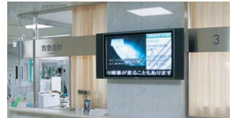
The Advanced Dual Picture Mode of the plasma display simultaneously shows hospital announcements and a background video from a DVD disc.
