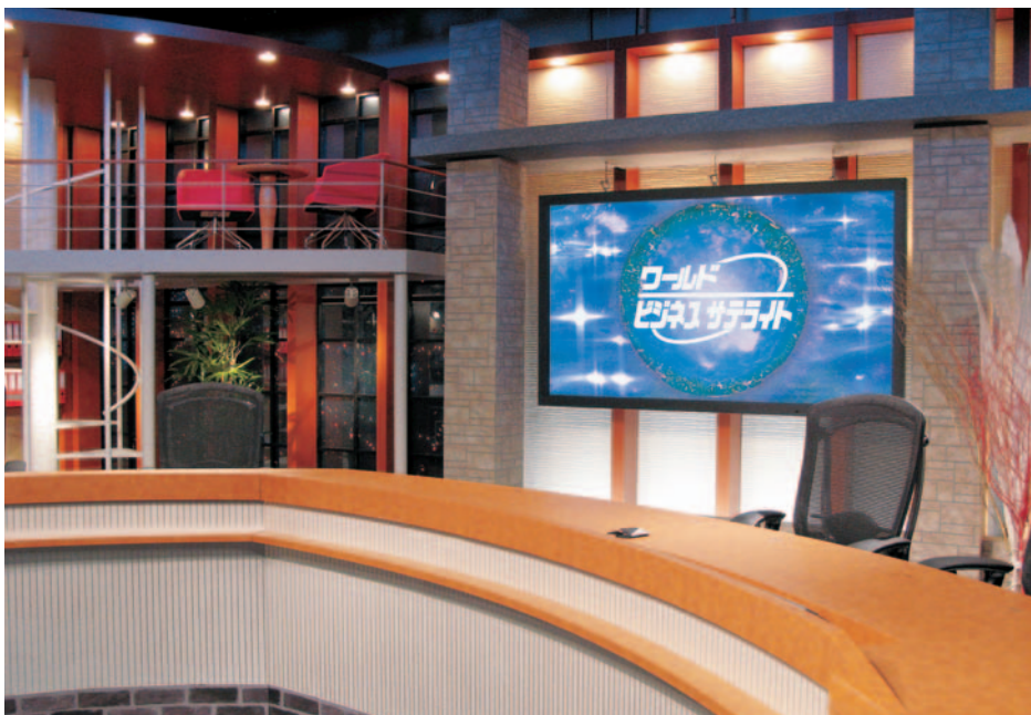
The 103-inch plasma display is positioned between the main newscaster and the commentator. When the studio is shown during programming, the display unit frequently appears on TV. This makes it essential that it have a large screen size and crystal-clear images.
